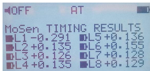
Reaction times generating an automatic false start (between -0.100s and +0.099s) are indicated in inverted video.
